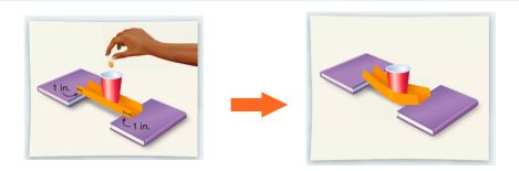
• Put two *new* strips of paper together to make a bridge with twice as many layers. Find the breaking weight for this bridge.
